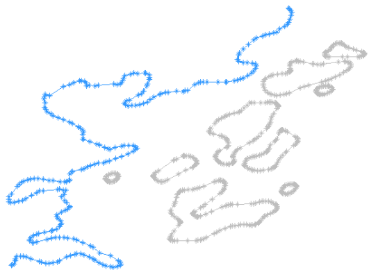
Figure 7: Input data for the second experiment. The blue contour is being generalized, while the grey closed contours represent the same bathymetric depth, but are located seaward of the target contour.
