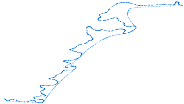
Figure 5: Intermediate stage of the generalization process. Note that the generalized (light blue) curve does not extend more seawards than the most seaward point of the original (dark blue) curve, but has removed extraneous detail from the landward side as expected. Note also the smoothness of the curve.
