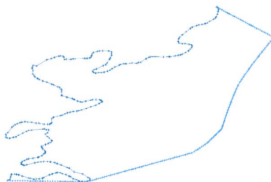
Figure 12: The final stage of generalization. All of the closed contours have been aggregated and generalized, so that the result (at much lower scale) preserves only the outer promontories of the originals, with smooth transitions between them.
