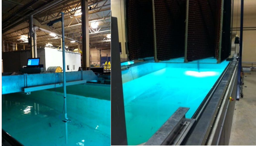
Figure 2: Experimental Setup for translational 3-D underwater experiments. (Left image) detector unit that includes a submerged fiber optic cable with a collimator that was connected to the spectrometer. (Right image) transmitting unit mounted to the wall of the tank.
