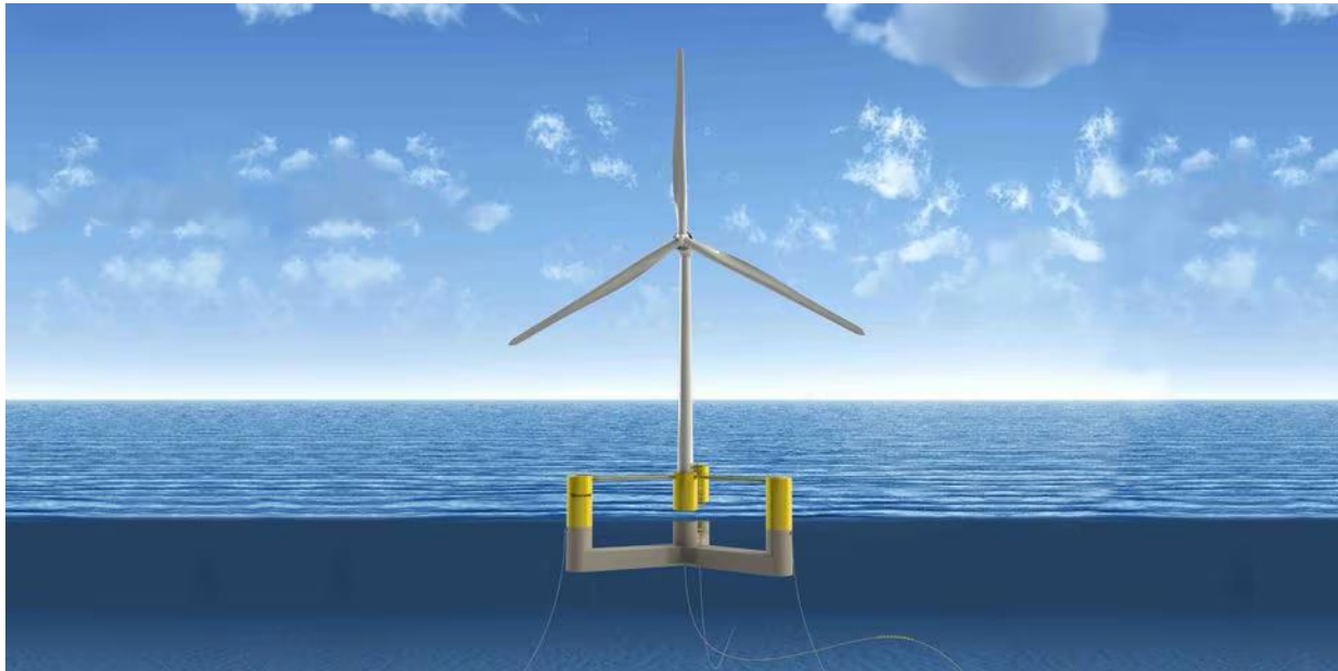
Figure 3.4.1 Design of the VoltturnUS (Abel, 2022)
