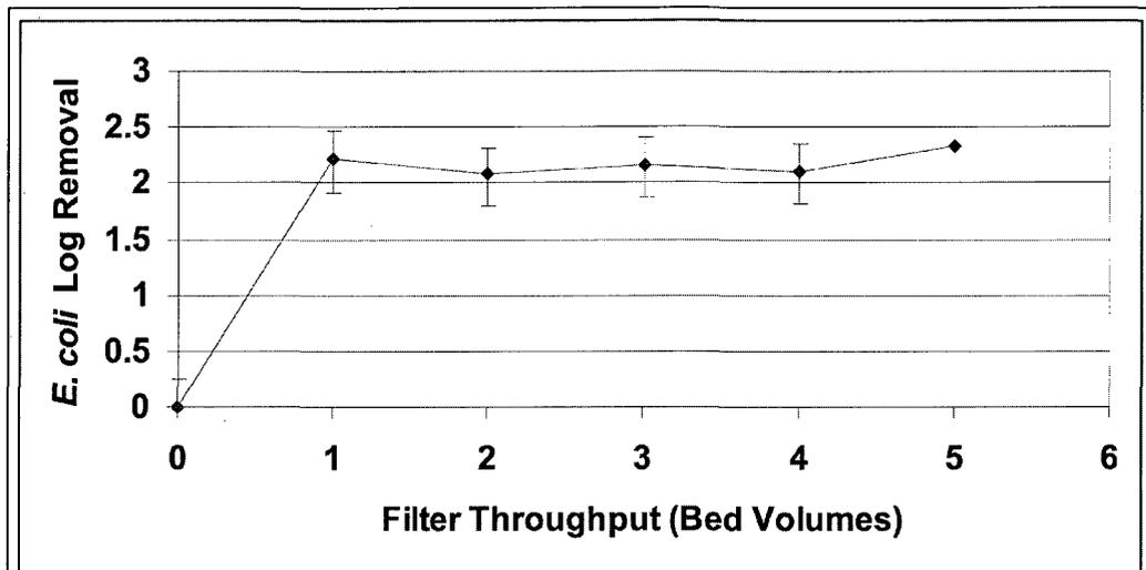
Figure 3.3 *E. coli* removal over time in a lab-scale experimental sand filter during continuous *E. coli* challenge at a concentration of  $1.33 \times 10^5$  / 100 mL. Steady state is reached before one bed volume (22.5 minutes) has been introduced (Unger, 2006).
