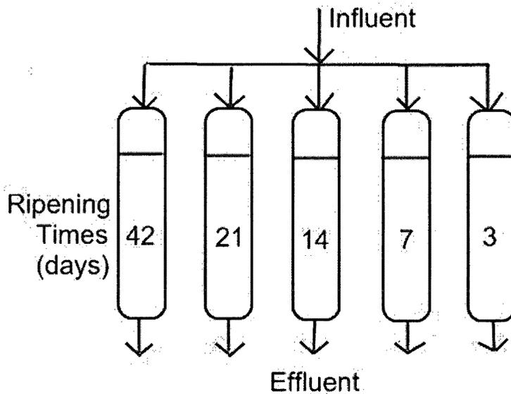
**Figure 3.1 Diagram of bench-scale ripening study filter arrangement.**
