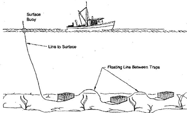
**Figure 1.1:** Passive fishing gear
