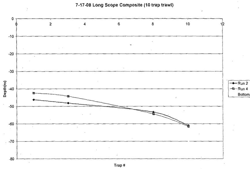
**Appendix A.16** Composite plot of 2 runs using a long-scoped end line as the towing hawser on a 10 trap trawl. Each colored line represents one series of towing data, and the line at the bottom represents the average water depth throughout this series of tows.
