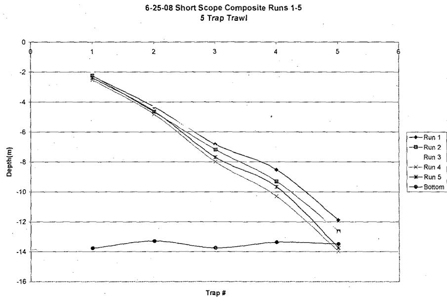
**Appendix A.2** Composite plot of 5 runs using a short-scope endline as the towing hawser on a 5 trap trawl. Each colored line represents one series of towing data, and the line at the bottom represents the average water depth throughout this series of tows.
