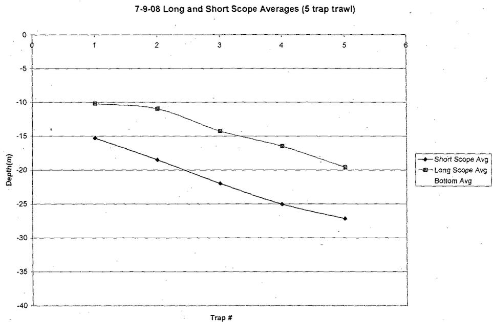
**Appendix A.11** Plot of the average of the long, and short-scope runs for a 5 trap trawl of the 7-9-08 day of testing.
