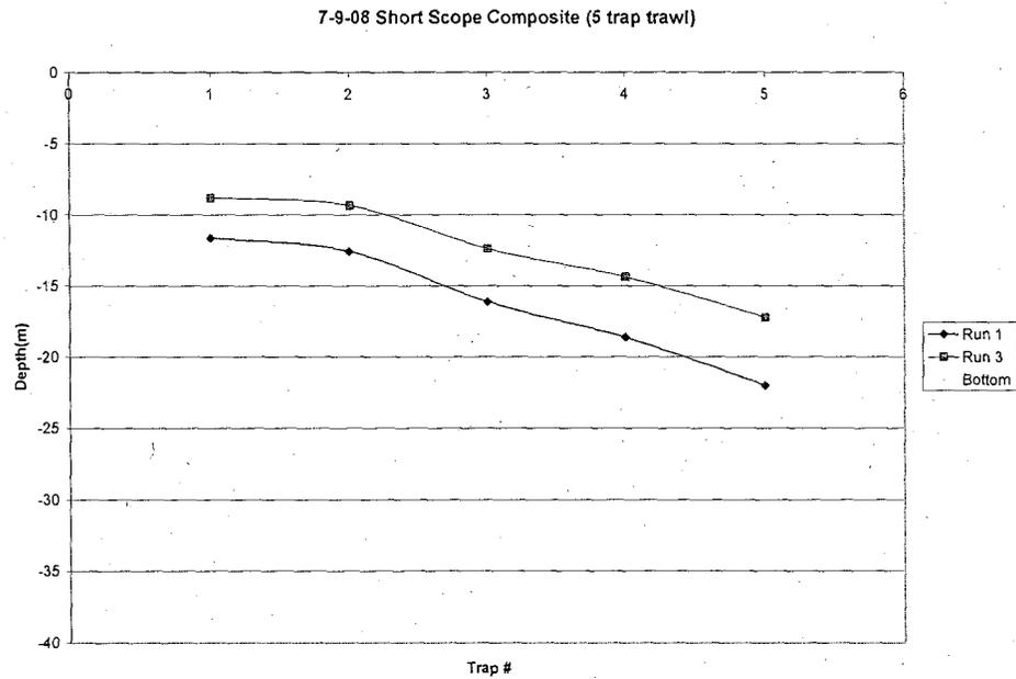
**Appendix A.9** Composite plot of 2 runs using a short-scoped end line as the towing hawser on a 5 trap trawl. Each colored line represents one series of towing data, and the line at the bottom represents the average water depth throughout this series of tows.
