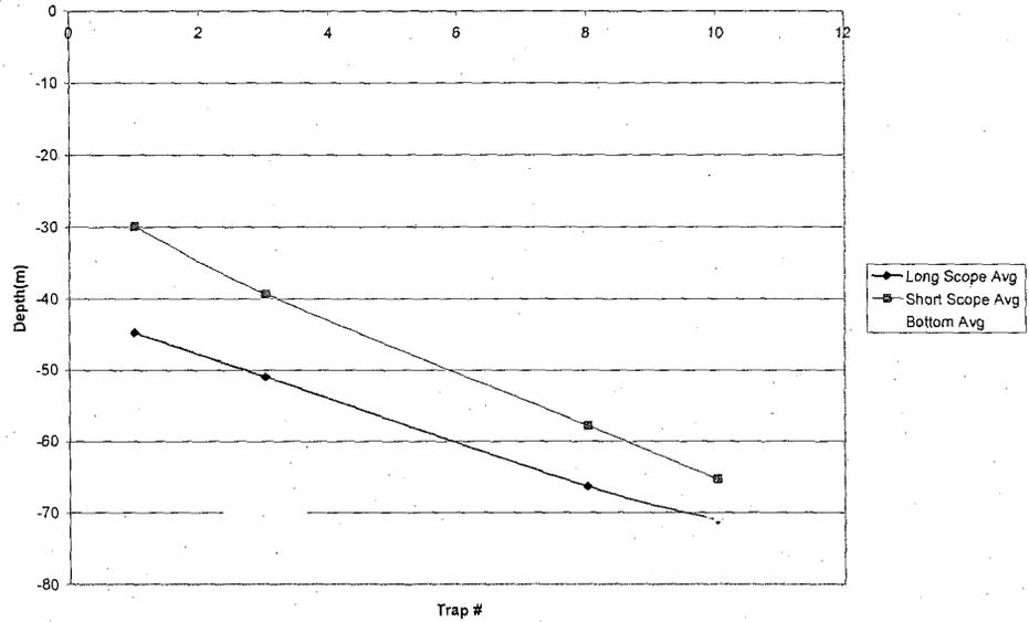
Appendix A.14 Plot of the average of the long, and short-scope runs for a 10 trap trawl of the 7-16-08 day of testing.
