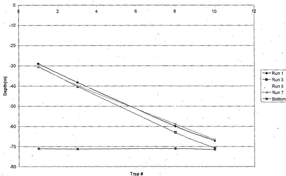
**Appendix A.12** Composite plot of 4 runs using a short-scoped end line as the towing hawser on a 10 trap trawl. Each colored line represents one series of towing data, and the line at the bottom represents the average water depth throughout this series of tows.
