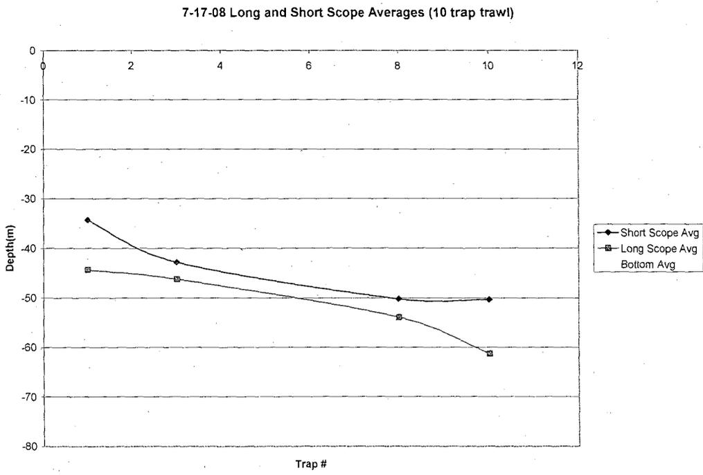
**Appendix A.17** Plot of the average of the long, and short-scope runs for a 10 trap trawl of the 7-17-08 day of testing.
