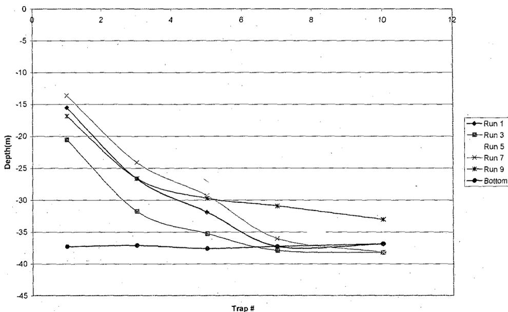
**Appendix A.6** Composite plot of 5 runs using a short-scoped end line as the towing hawser on a 10 trap trawl. Each colored line represents one series of towing data, and the line at the bottom represents the average water depth throughout this series of tows.
