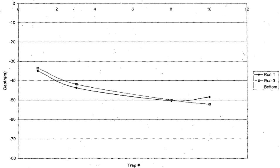
Appendix A.15 Composite plot of 2 runs using a short-scoped end line as the towing hawser on a 10 trap trawl. Each colored line represents one series of towing data, and the line at the bottom represents the average water depth throughout this series of tows.
