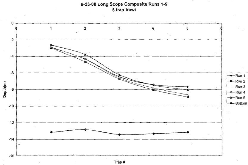
**Appendix A.1** Composite plot of 5 runs using a long-scope endline as the towing hawser on a 5 trap trawl. Each colored line represents one series of towing data, and the line at the bottom represents the average water depth throughout this series of tows.
