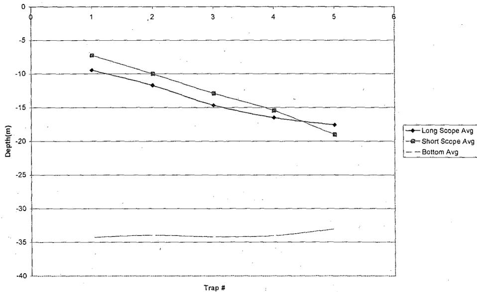
**Appendix A.5** Plot of the average of the long, and short-scope runs for a 5 trap trawl of the 6-25-08 day of testing.
