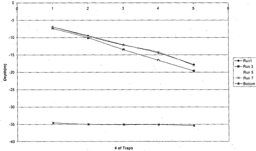
**Appendix A.4** Composite plot of 5 runs using a short-scoped end line as the towing hawser on a 5 trap trawl. Each colored line represents one series of towing data, and the line at the bottom represents the average water depth throughout this series of tows.
