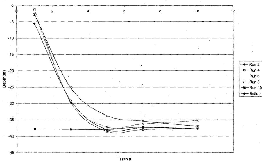
**Appendix A.7** Composite plot of 5 runs using a long-scoped end line as the towing hawser on a 10 trap trawl. Each colored line represents one series of towing data, and the line at the bottom represents the average water depth throughout this series of tows.
