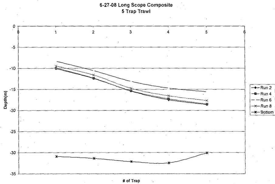
**Appendix A.3** Composite plot of 5 runs using a long-scoped end line as the towing hawser on a 5 trap trawl. Each colored line represents one series of towing data, and the line at the bottom represents the average water depth throughout this series of tows.
