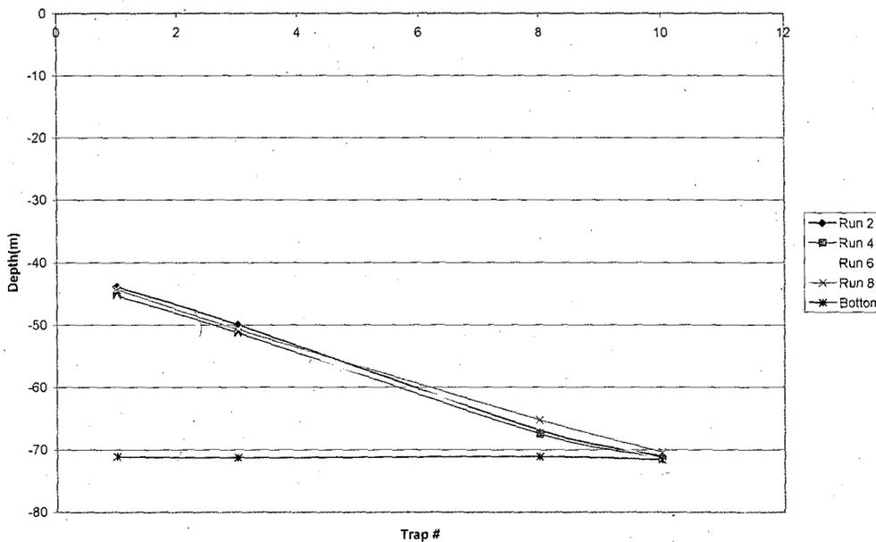
**Appendix A.13** Composite plot of 4 runs using a long-scoped end line as the towing hawser on a 10 trap trawl. Each colored line represents one series of towing data, and the line at the bottom represents the average water depth throughout this series of tows.
