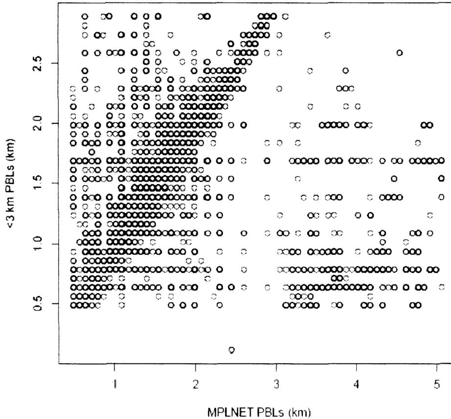
Figure 6. Comparison between PBL heights calculated by MPLNET for its level 1.5b data set vs. PBL heights calculated for the lowest 3 km of the atmosphere. Scatter beyond the downward adjustment of PBL heights above 3 km is due to the sensitivity of the wavelet covariance transform to the amount of data in the starting lidar backscatter profile, i.e. the depth of atmosphere for which the PBL is calculated.
