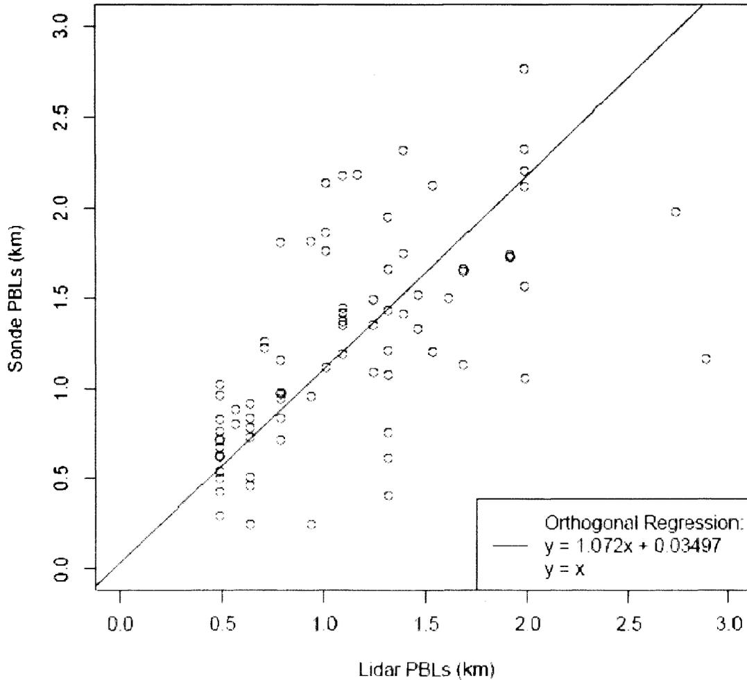
Figure 8. Orthogonal regression between lidar-derived PBL heights and sonde-derived PBL heights. The 1:1 line is shown in dotted gray for comparison.
