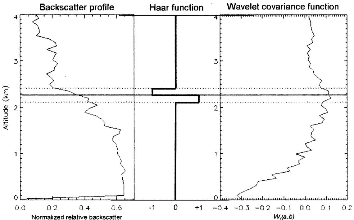
Figure 4. An example 1-minute backscatter profile, the matching Haar wavelet, and the wavelet covariance transform used to identify the planetary boundary layer height. The solid gray line marks the maximum of  $W_f(a,b)$ , while the dashed lines show the dilation  $a$  of the Haar function.
