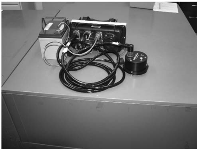
Figure 2. The IRIS/PASSCAL broadband stations used in this project consisted of an Episensor accelerometer and an RT-130 recorder, powered by a 12 volt battery. (Any use of trade names is for descriptive purposes only and does not imply endorsement by the U.S. government.) These units were housed in steel security boxes bolted to the floors in small alcoves.
