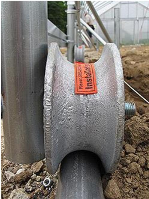
**THE MOVABLE TUNNEL USES HEAVY-DUTY WHEELS WITH BEARINGS THAT GLIDE OVER EXTENDED RAILS.**
