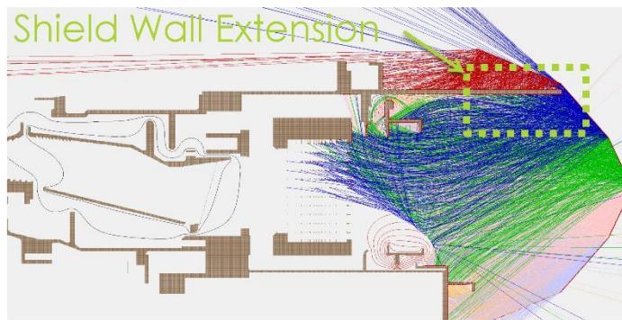
Figure 7: This shows the outer wall extension blocking many of the angular distribution on ions that were previously impacting the conversion surface
