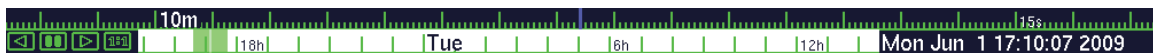
Fig 1: The GeoZui4D time bar. The top section animates as time passes. The lower section gives an overview.
