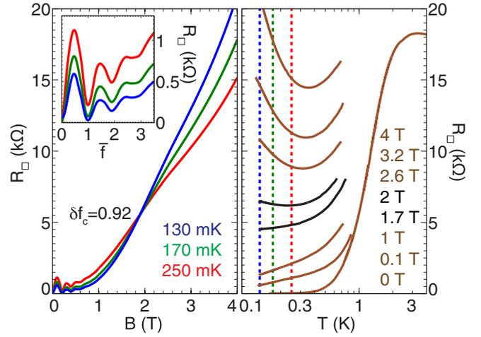
FIG. 2. (Color online) A high field SIT. Film on NHC2 with  $R_N = 17$  k $\Omega/\square$ . (a) Isothermal magnetoresistance curves at 130, 170, and 250 mK show a single crossing at  $B_c = 1.9$  T. Inset: Expanded low field region. (b)  $R_{\square}(T)$  at discrete magnetic fields spanning  $B_c$ . Vertical dashed lines indicate the isothermal slices in (a).
