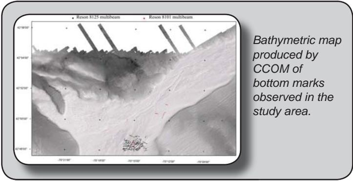
*Bathymetric map produced by CCOM of bottom marks observed in the study area.*
