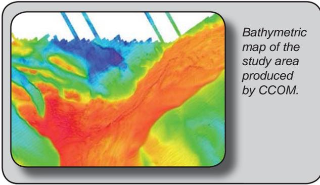
MBES) was used in 2003. It allowed enhanced resolution (up to one meter) covering a 2 x 3 km area in the middle of the study site. Both MBES surveys were conducted to provide coverage over both the open and closed areas in the western GOM. About 25 km of sidescan transects were collected in 2003 overlapping the previously collected MBES data. A bottom videographic survey of over 189 bottom sampling sites (collected by Larry Ward, UNH) was also analyzed during this study.
