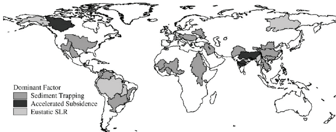
Fig. 3 Dominant factor determining the estimate of baseline ESLR for each of the 40 deltas. Sediment trapping is the dominant factor for 27 deltas, eustatic sea-level rise is most important for eight deltas and accelerated subsidence predominates in five deltas. This assessment identifies the major factor at play under contemporary baseline conditions .
