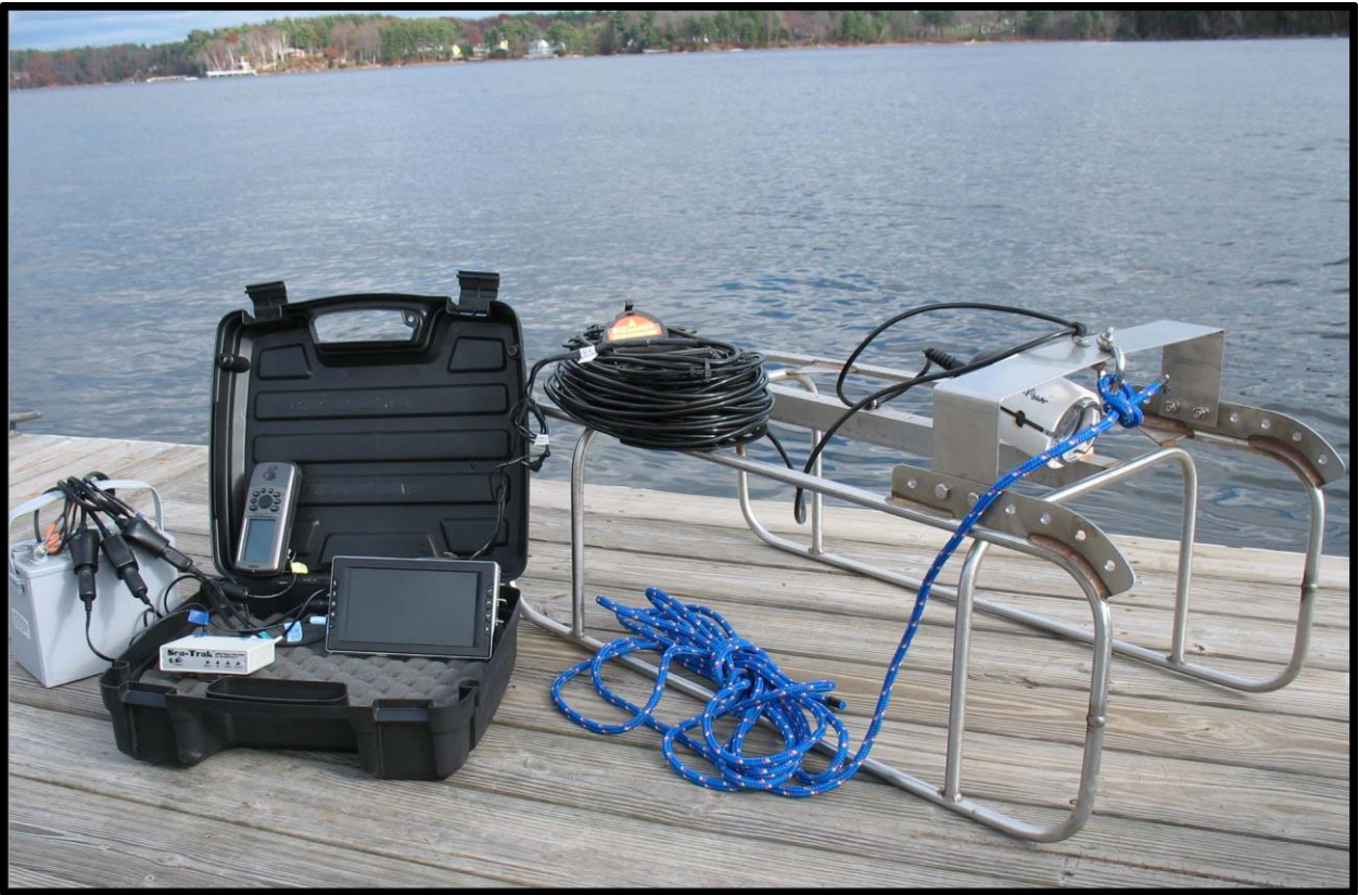
Fig. 3. Towed underwater video system showing major components (see text for details).
