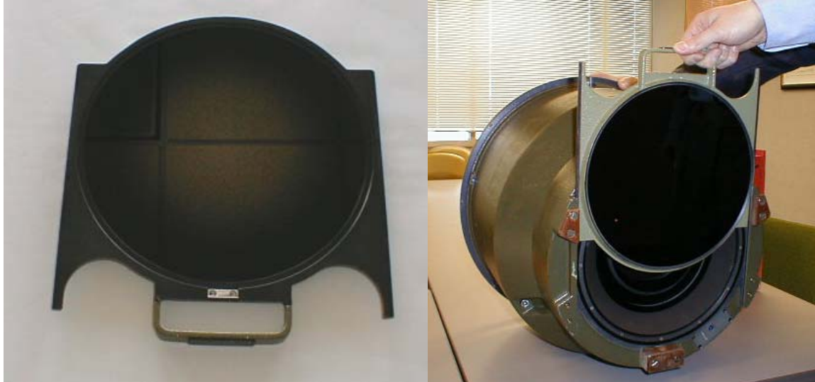
Figure 1. Left: Long wavepass filter for B&WIR photography. Right: Installing the filter on the Wild RC30 lens cone.
