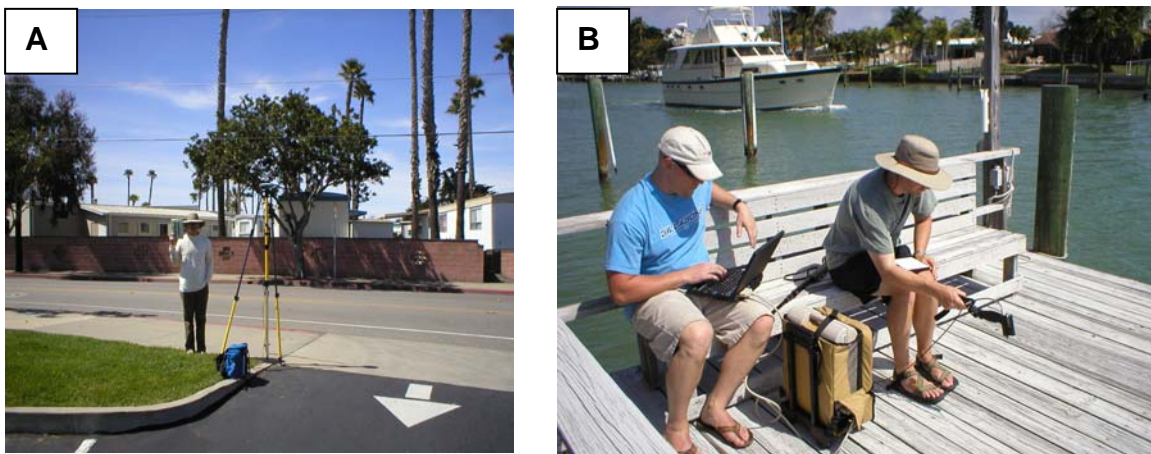
Figure 2. a) collecting the GPS position of well defined points in St. Pete Beach, Florida b) collecting spectral signatures of features along the coastline using an ASD
