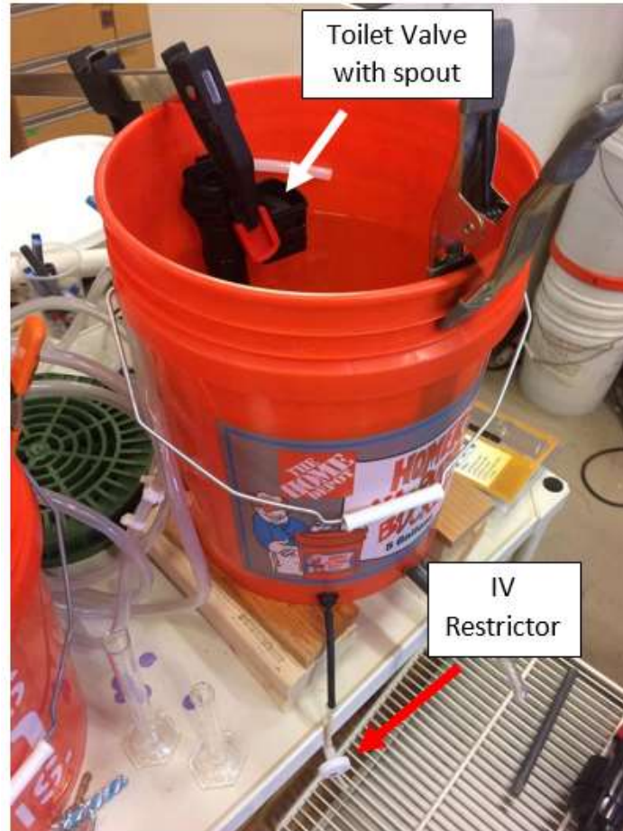
Figure 3: Photo of dosing reservoir with a toilet valve for water level control and IV restrictor for outlet flow control.
