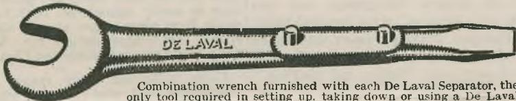
Combination wrench furnished with each De Laval Separator, the only tool required in setting up, taking down or using a De Laval machine, the simplest as well as the best cream separator ever built.
