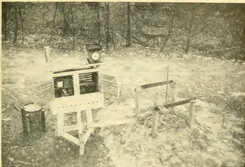
Fig. 1. Maple Seed Storage Experiment. Shows weather recording instruments as well as method of storing seeds in cloth bag, in bucket of sand, under leaf litter, and stratified under two feet of sand.
