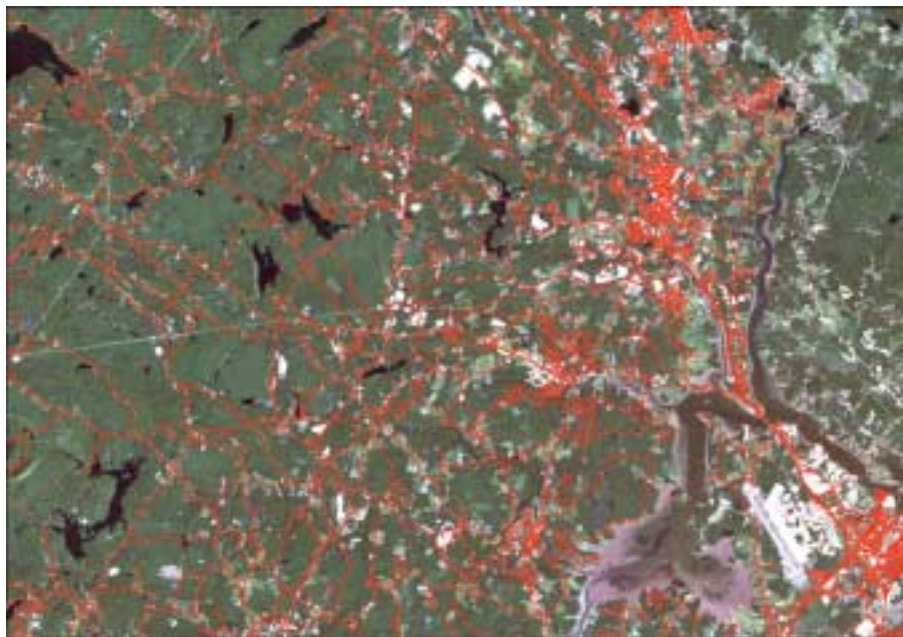
Figure 2. Georeferenced Subset of Landsat 5 Thematic Mapper Image (bands 3, 2, 1 – acquired 9/8/90) for an area around Great Bay. Red vectors represent NH Department of Transportation road centerline data overlain on the source imagery.
