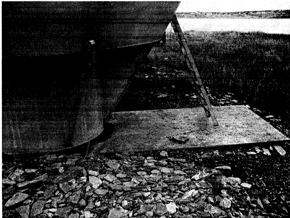
Figure 7.8: Buoy launch plate placed under the buoy. Steel rods shown under buoy are to allow the buoy to roll into the ocean during launch.
