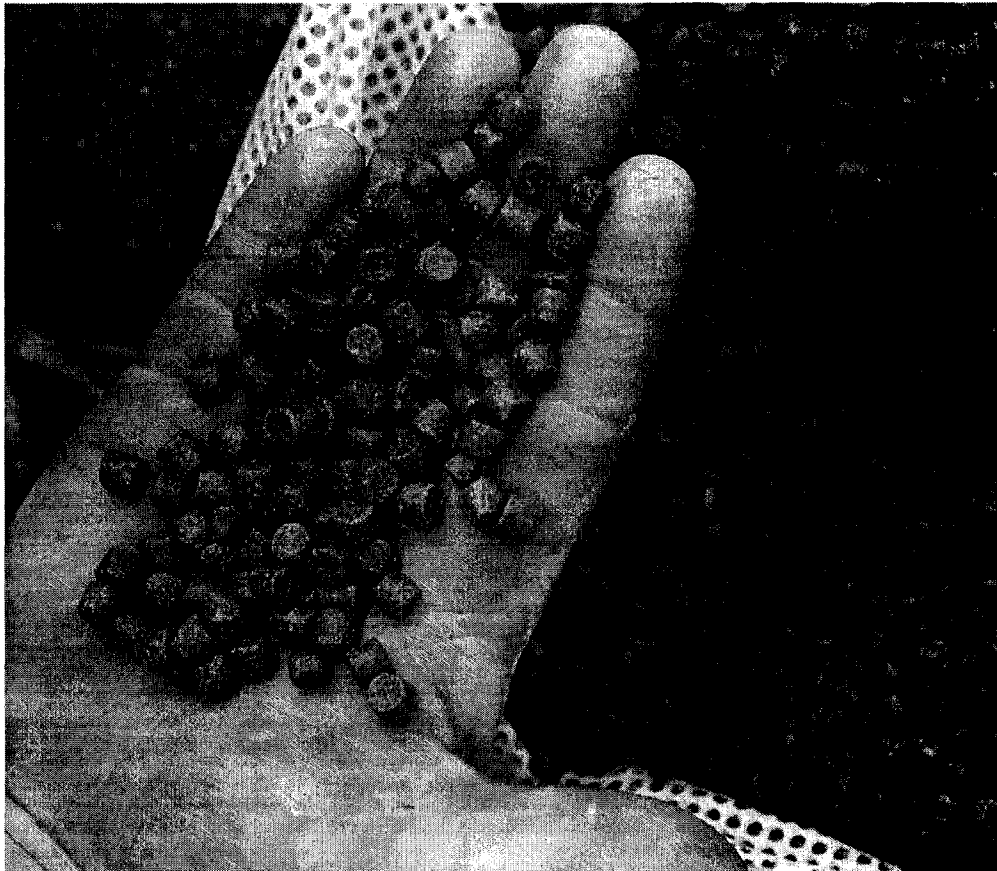
Figure 3.10: Feed, 8 millimeter, after being pumped through the mixing chamber and Hidrostal fish pump.
