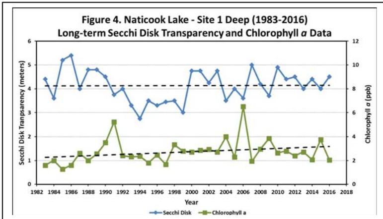
Figures 4 and 5. Changes in the Naticook Lake water clarity (Secchi Disk depth), chlorophyll *a*, dissolved color, and total phosphorus concentrations measured between 1983 and 2016. **These data illustrate the relationship among plant growth, water color, and water clarity. Total phosphorus data are also displayed and are oftentimes correlated with the amount of plant growth.**
