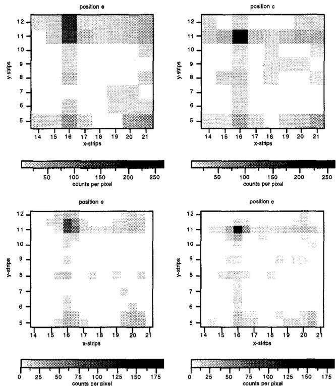
Fig. 3a. Image of  $170 \mu\text{m}$  diameter 122 keV beam.
