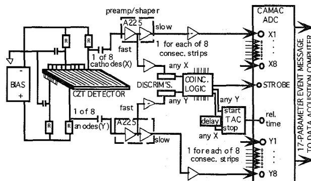
Figure 1. Test setup (orthogonal stripe coincidence mode)
