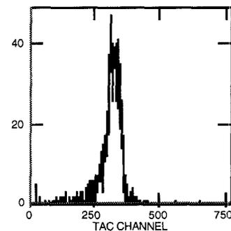
Fig. 9. Relative cathode-anode signal arrival time. FWHM = 270 ns.
