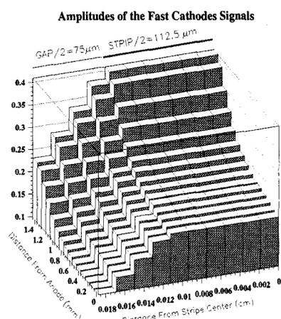
Fig. 8a. Cathode signal simulation
