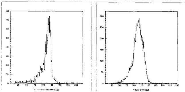
Fig. 2a. 122 keV single “pixel” spectrum
