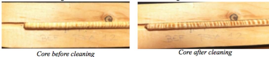
Figure 2: The core on the left was not cleaned with a razor, while the core on the left was cleaned for easier reading.
