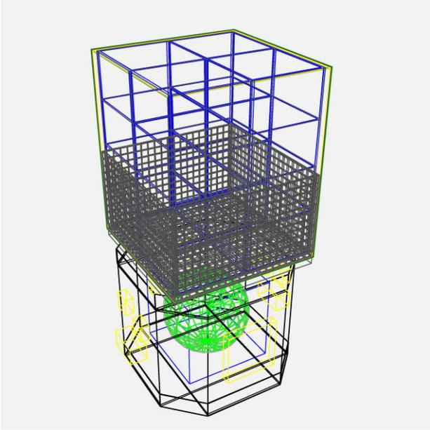
Fig. 2. ACT mass model used for MGGPOD simulations. It consists of a Xe gas tracker surrounded by a LaBr<sub>3</sub> scintillator calorimeter.
