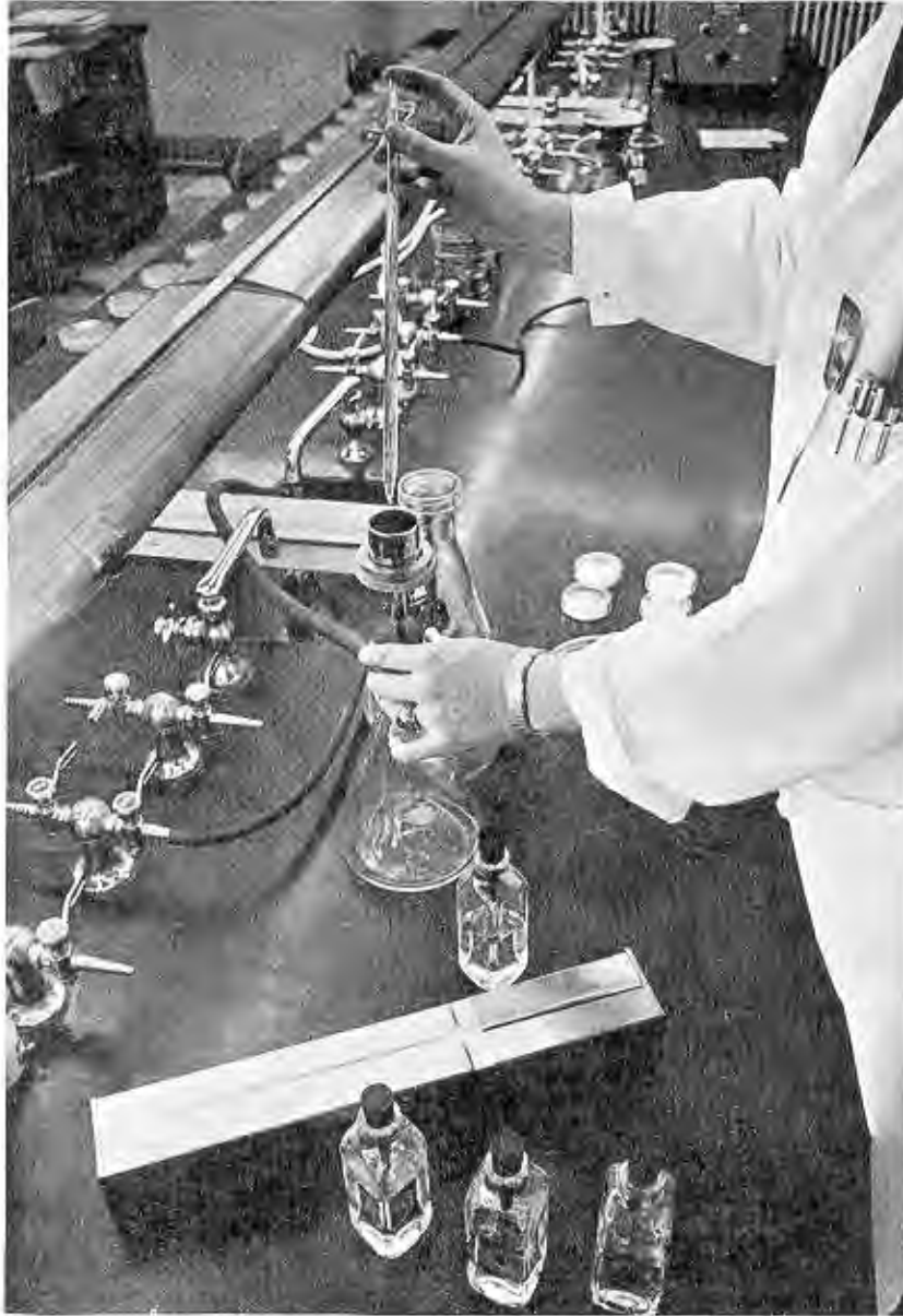
Figure C. Membrane filter tests for coliforms.
