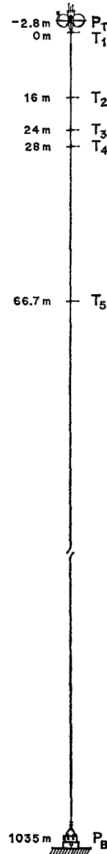
FIG. 4. A typical array (JOSIE 175 SW), showing sensor depths relative to T_1 (see Table 1 for other installations). Eighteen 10-inch diameter glass spheres (not shown) were attached to the cable for buoyancy.
