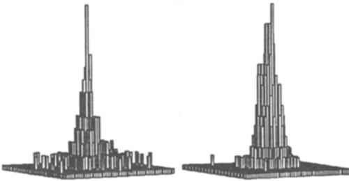
**Figure 5.** Compton (left) and Pair Images (right) at 25 MeV.
