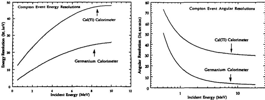
Figure 3. TIGRE energy and angular resolutions for Compton events.
