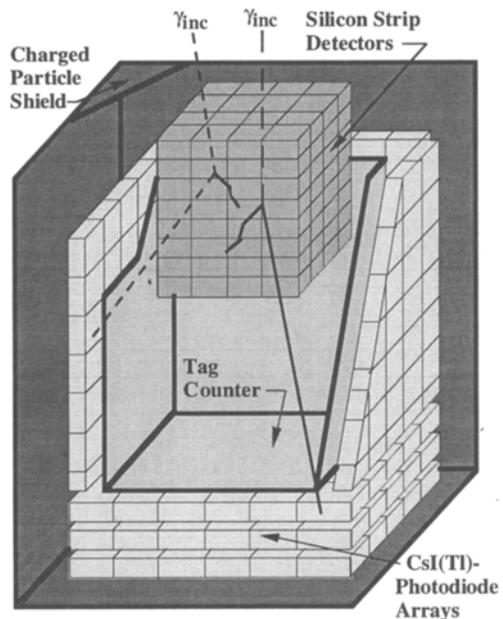
**Figure 1.** Tracking and Imaging Gamma Ray Experiment (TIGRE)
