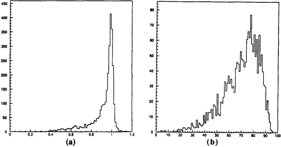
Figure 2. Total detected energy loss for a) 1 MeV and b) 100 MeV incident photons
