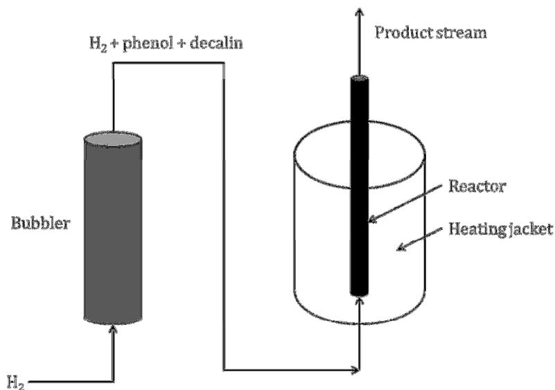
Figure 4. Reactor schematic
