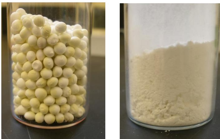
Figure 2. Prepared Mo-gamma alumina (left) and Mo-Y-zeolite (right)
