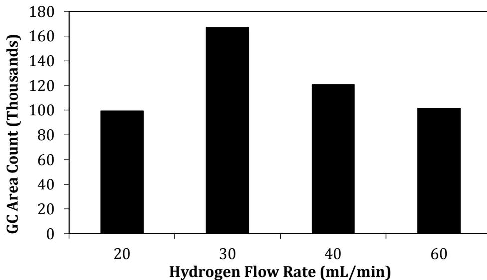
Figure 3. Calibration of hydrogen flow rate through bubbler
