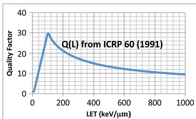
**Figure 1.** Quality factors are directly linked to linear energy transfer (LET). By directly measuring LET, the CRaTER instrument is able to provide a direct connection between measurements and biological impact via the quality factor.
