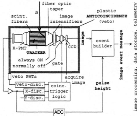
FIGURE 2. Complete instrument functional and logic diagram.
