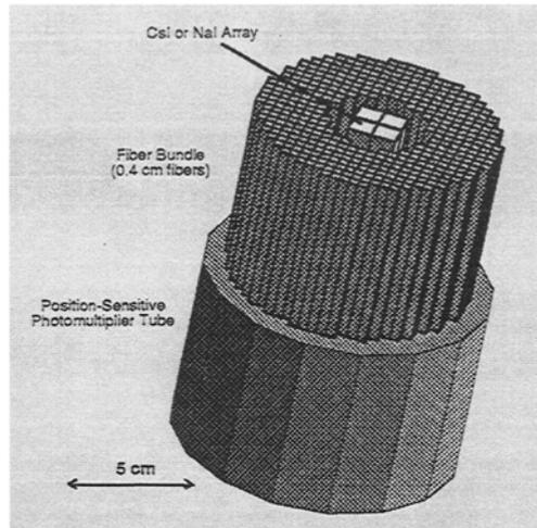
**FIGURE 3.** Schematic diagram of a polarimeter module.
