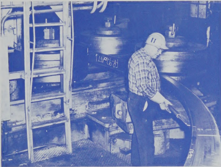
In the construction of four submarines at the Portsmouth Naval Shipyard, $900,000 have been saved through this frame fabrication method.
