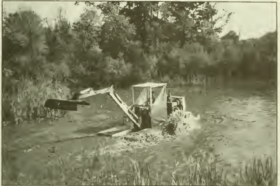
In August Aquatic Control Technology used the "Muck Mess Monster", a hydrorake, to clean out the overabundant weeds in the Mill Pond.
