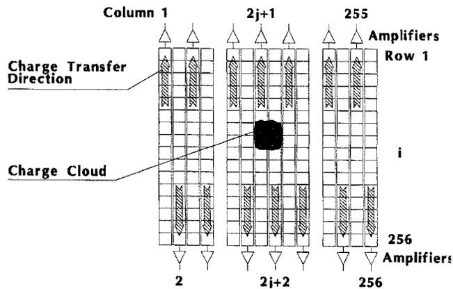
FIGURE 2. Schematic view of the Bi-Directional CCD.
