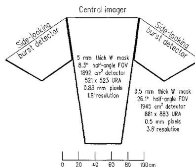
**FIGURE 1.** Schematic of the MARGIE  $\gamma$ -ray telescope.
