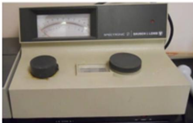
Figure 4.1: Bosch and Lomb Spectronic 21 spectrophotometer used for turbidity measurements during this projects.
