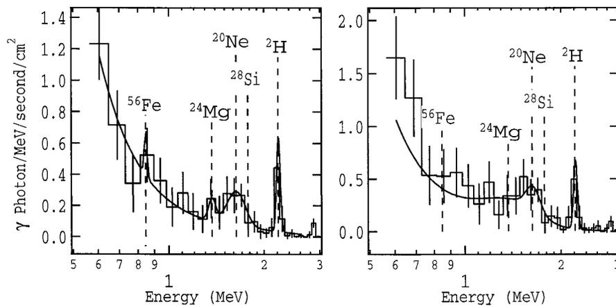
**FIGURE 3.** COMPTEL spectra of the *whole event* (left) and the *impulsive phase* (right). The solid lines are fits made up of a power law and either 3 or 5 gaussians. Typical nuclear lines are marked.
