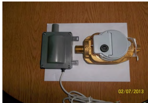
New Residential Meter and Transponder
