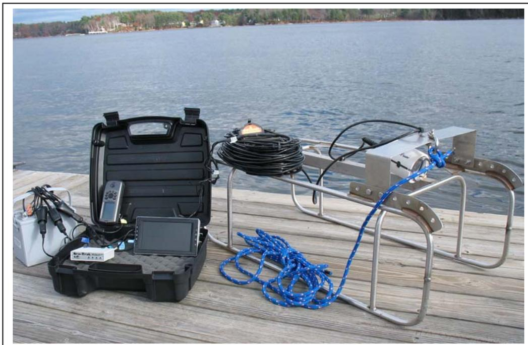
Fig. 2. Towed underwater video system showing major components when deployed in sled mode (see text for details).
