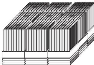
**FIGURE 5.** An array of nine GRAPE modules.
