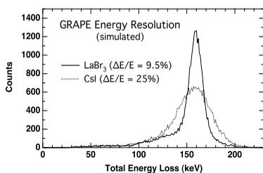
**FIGURE 4.** Simulated results showing the improved energy resolution that would result from changing the CsI calorimeter to one made from LaBr<sub>3</sub>.
