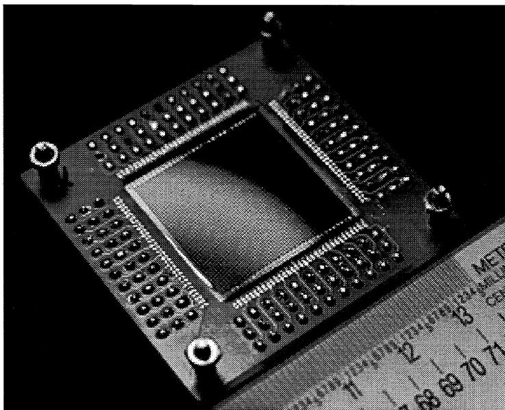
Figure 4. Photo of UNH prototype CZT strip detector.
