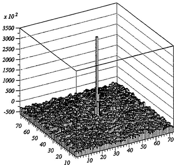
Figure 10. Reconstructed image based on test results with optical light beam illuminating 71 x 73 test mask. Signal is observed with 8" x 11" (127  $\mu$ m pixel pitch) amorphous silicon detector array from Xerox Palo Alto.
