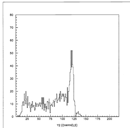
Figure 6. Spectrum of <sup>57</sup>Co (122 keV) as measured from a single 375 μm pixel.
