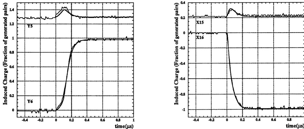
**Figure 4.** Measured and simulated electron signals on two neighboring anodes (Y5 and Y6) and cathodes (X15 and X16) due to alphas incident on the cathode plane in the center of anode Y6 (left) and in the center of cathode X16 (right).
