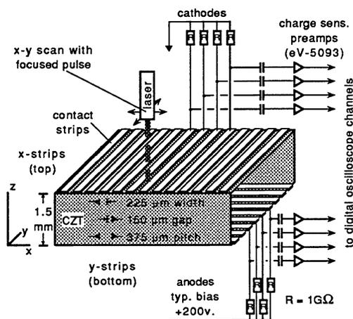
Figure 2. Small segment of the prototype strip detector.
