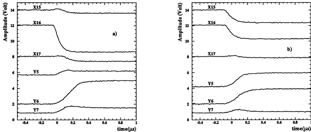
**Figure 3.** Electron charge signals on three contiguous anodes and three contiguous cathodes with a) the laser centered on cathode X16 and anode Y6 and b) the laser in the center of the gap between cathodes X15 and X16 and between anodes Y5 and Y6.
