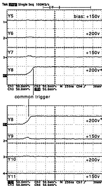
**Figure 11.** Anode signals from a sample event. Signals from seven contiguous anode strips triggered by the signal on the central collecting strip (Y8). A  $^{137}\text{Cs}$ , 662 keV, gamma source was used..
