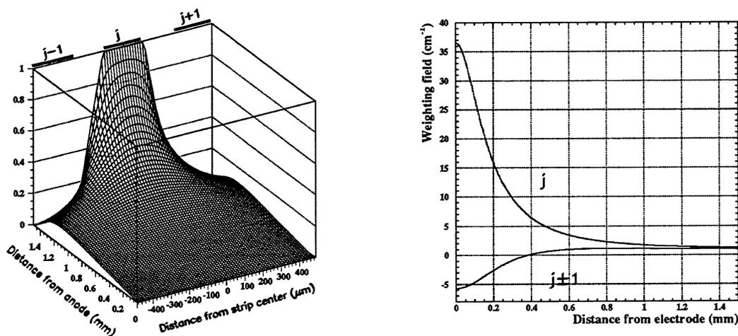
**Figure 1.** Left: The cathode weighting potential. Right: The weighting field as a function of the distance from an electrode along an axis centered on the electrode  $j$  and along an axis centered on its neighbor  $j \pm 1$ .
