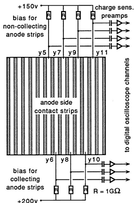
**Figure 10.** Coplanar anode setup for strip detector test. Signals from seven contiguous anode strips are monitored with digital oscilloscopes. Even numbered anode strips (collecting) are biased at +200 V, odd numbered anode strips are biased at +150 V. Cathode strips (not shown) are biased at ground potential.
