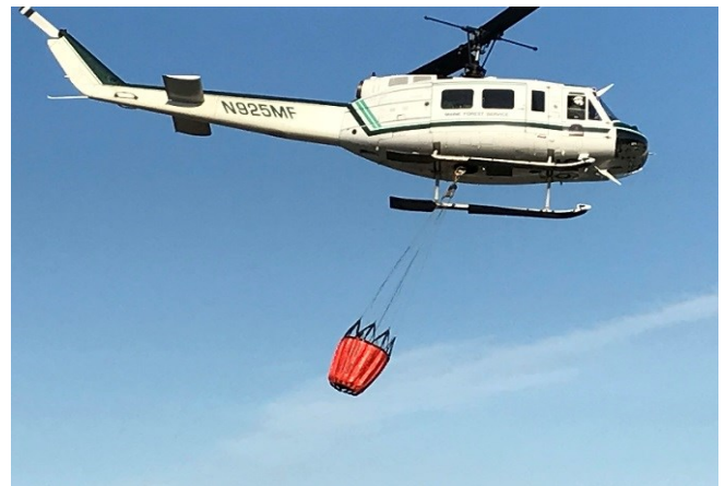
The Maine Forest Service helicopter with a water basket used for fighting forest fires
