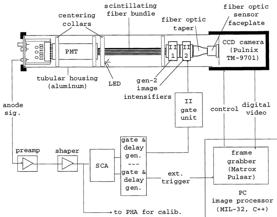
Figure 7. Schematic diagram of the SONTRAC prototype.
