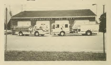
In the year 2002, the Town took delivery of the new Smeal fire engine replacing the 1970 American LaFrance fire engine. The engine arrived in April and was placed in service in June, after two months of training by the members of the department. The truck carries 1,500 gallons of water and has a pumping capacity of 1,250 gallons of water a minute and carries 5 firefighters.
