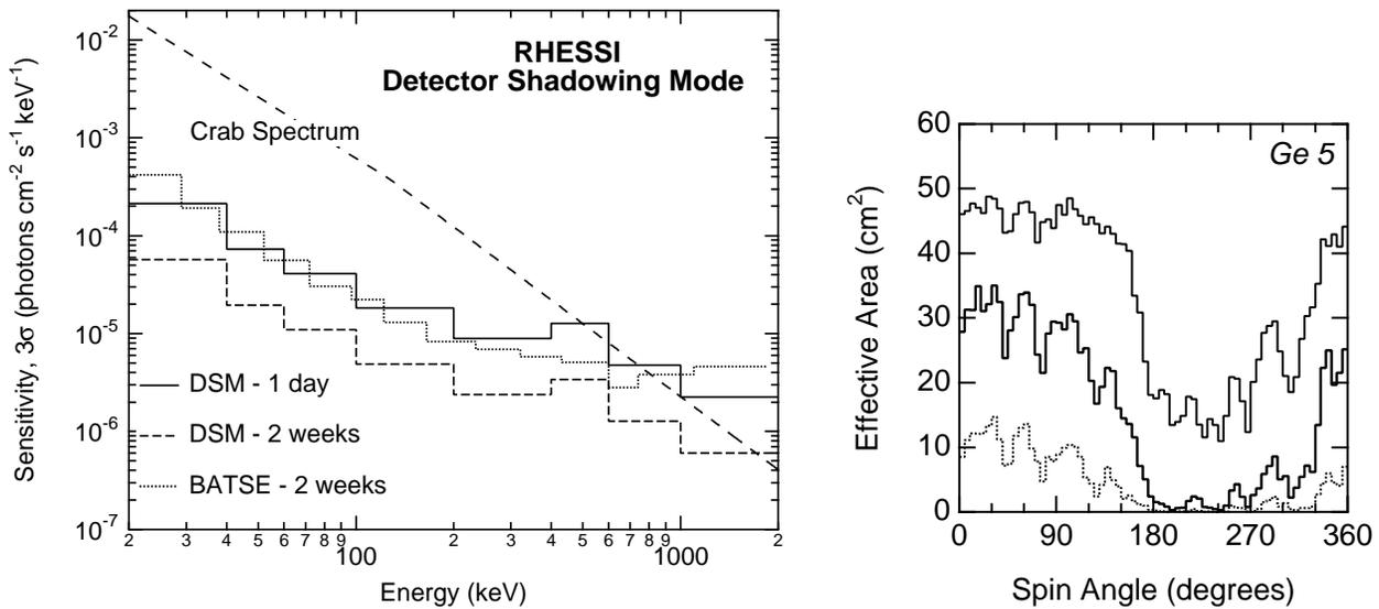
**Figure 6.** Left: continuum sensitivity for monitoring of sources using RHESSI in the Detector Shadowing Mode, with the BATSE EOM sensitivity and the spectrum<sup>16</sup> of the Crab (nebula plus pulsar) for comparison. Right: Modulation pattern (effective area versus azimuth angle) expected for one of the RHESSI detectors for a cosmic source in the detector plane at 100 keV, 50 keV, and 30 keV (top to bottom).
