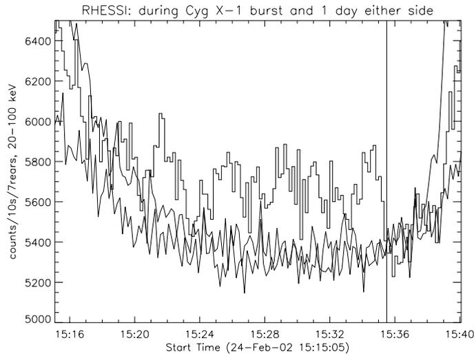
**Figure 5.** Occultation step of Cygnus X-1 on February 24, 2002. The histogram shows the data on February 24 during the outburst of the source. The other two traces are 15 orbits (about 1 day) before and after. The vertical line marks the time at which the source set (derived from the spacecraft ephemeris and the known source position, not the rate data themselves). At the beginning and end of the plot the spacecraft is in regions of higher background further from the Earth's magnetic equator.
