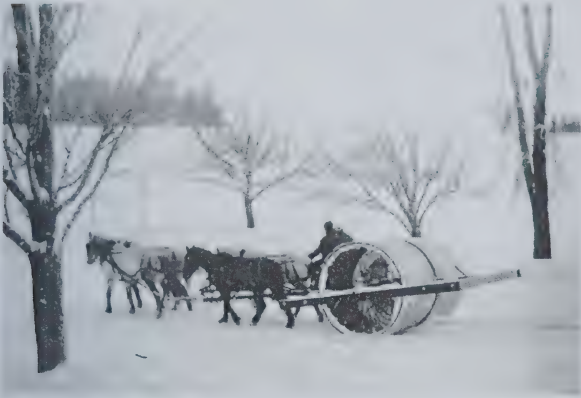
1925 Snow roller (photo taken on Harry Harmon's porch now known as the Wells property)
