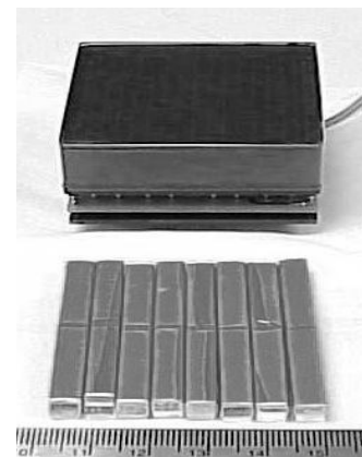
Figure 4: The Hamamatsu H8500 MAPMT (top), and several plastic scintillator elements (bottom).
