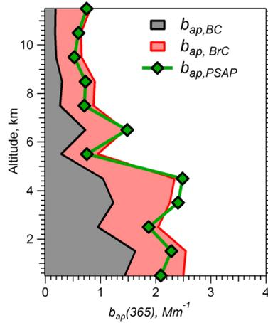
**Figure 2.** Vertical profiles of estimated black carbon (BC) and BrC absorption coefficients, along with the inferred ambient aerosol observed total absorption (PSAP), all at 365 nm. Uncertainty associated with each parameter was 45% for  $b_{ap,BrC}(365)$ , 22% for  $b_{ap,BC}(365)$ , and 29% for  $b_{ap,PSAP}(365)$  (details in supporting information).
