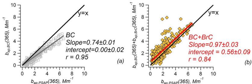
**Figure 3.** Closure analysis of absorption coefficients at 365 nm between (a) BC and (b) the sum of BC and BrC, each compared to total aerosol absorption from PSAP data. Orthogonal distance regression fit results are shown.
