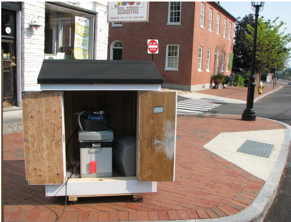
Photo 3: This shows how the influent was collected via a deep sump catch basin and drawn into a sampler. The location is represented by the blue dot in figure 1.
